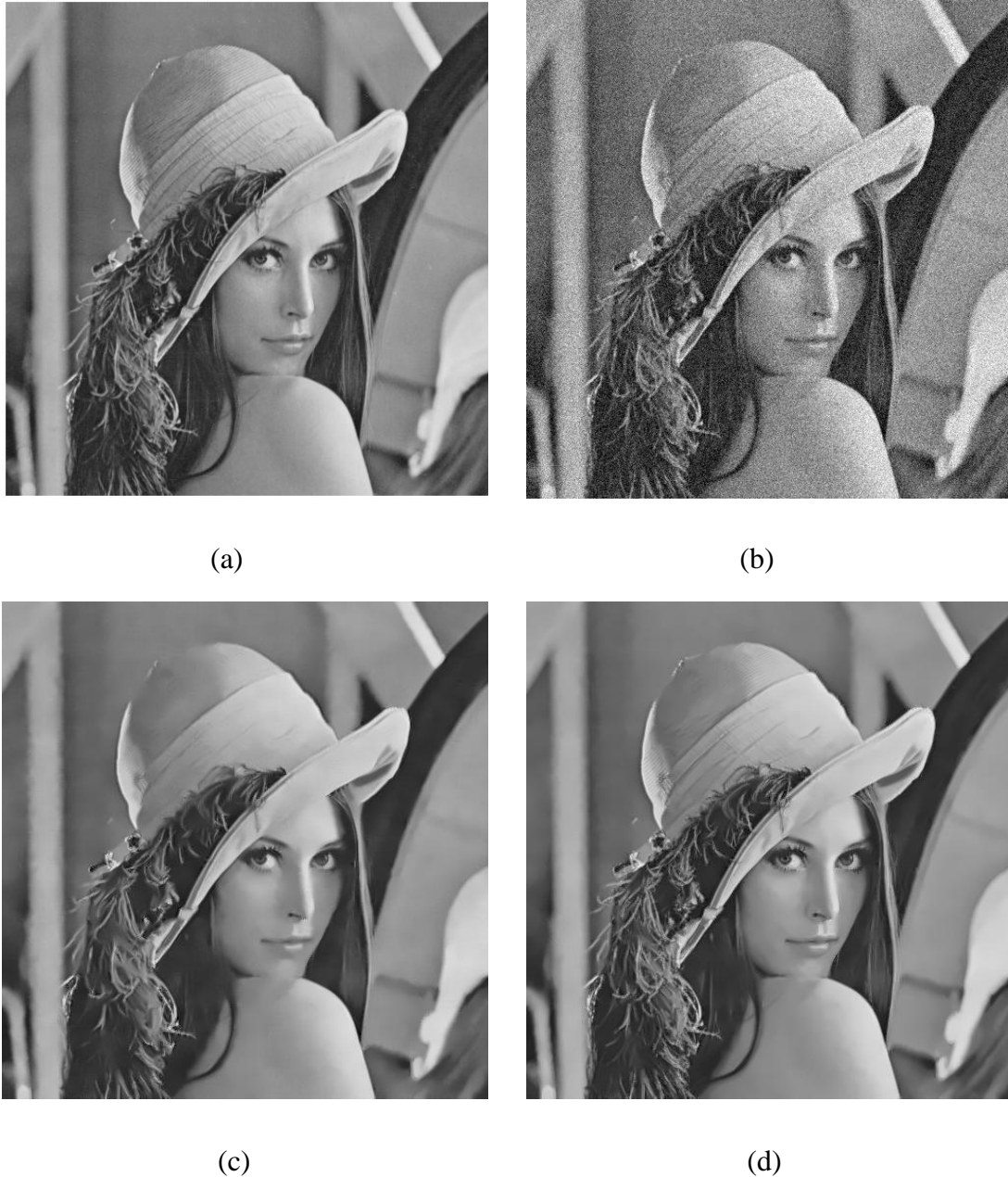
Figure 4- 6: Subjective comparison for denoising performance for Non-Local Means at noise level \sigma=20 . (a) Noise free image Lena, (b) noisy image with Additive white Gaussian noise, (c) denoised image using the NLM method, PSNR= 31.89, and (d) denoised image using the proposed method, PSNR = 33.32.
